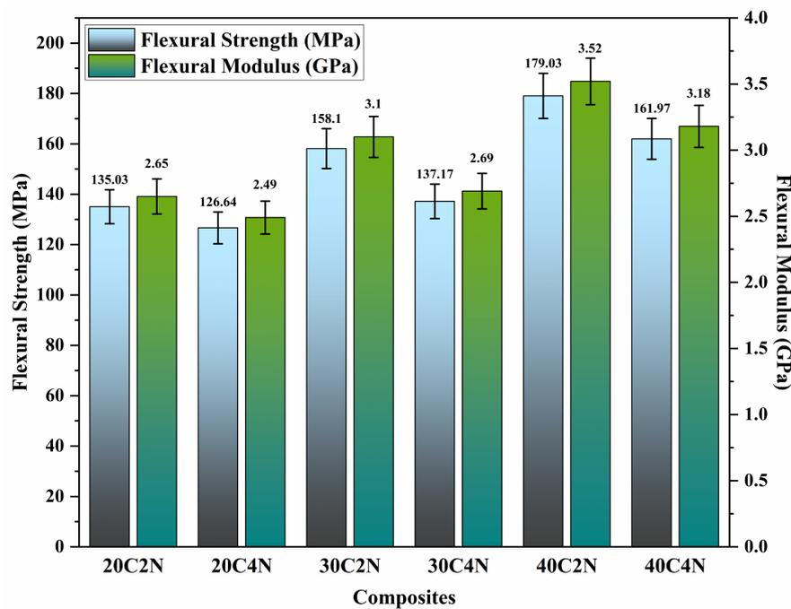
Figure 9. Flexural properties of the coir fiber nanoclay-reinforced epoxy composites.
