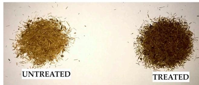
Figure 2. Chopped alkaline-treated and untreated coir fibers.
