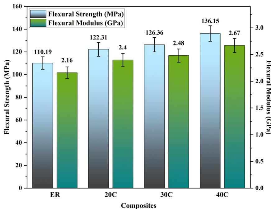
**Figure 8.** Flexural properties of the coir fiber-reinforced epoxy composites.
