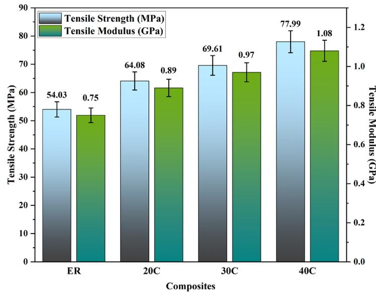
Figure 5. Tensile properties of the coir fiber-reinforced epoxy composites.
