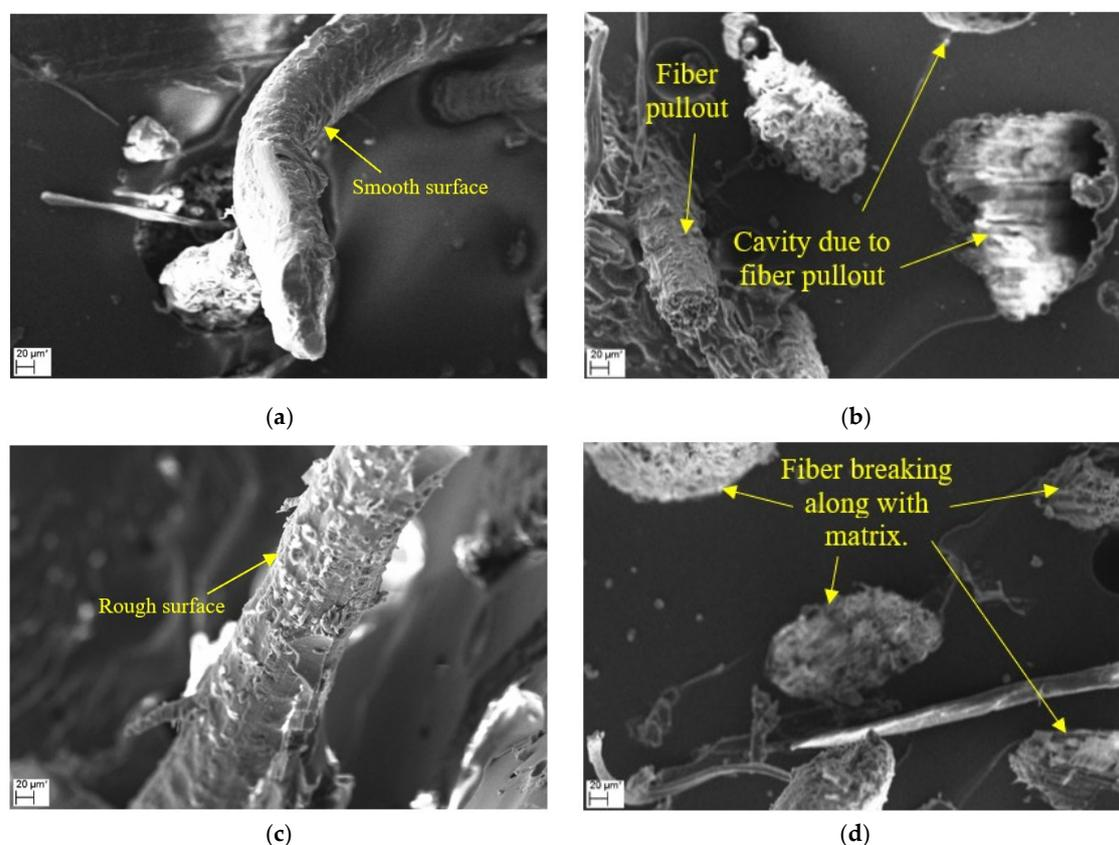
**Figure 4.** SEM images of the fractured surface of the (a,b) 20UC and (c,d) 20C composites.
