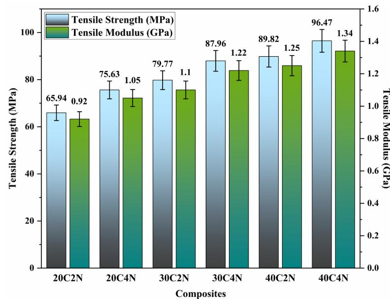
Figure 6. Tensile properties of the coir fiber and nanoclay-reinforced epoxy composites.
