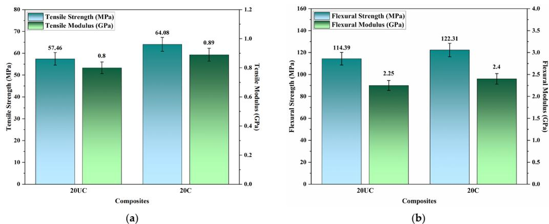
Figure 3. (a) Tensile and (b) flexural properties of the 20UC and 20C composites.
