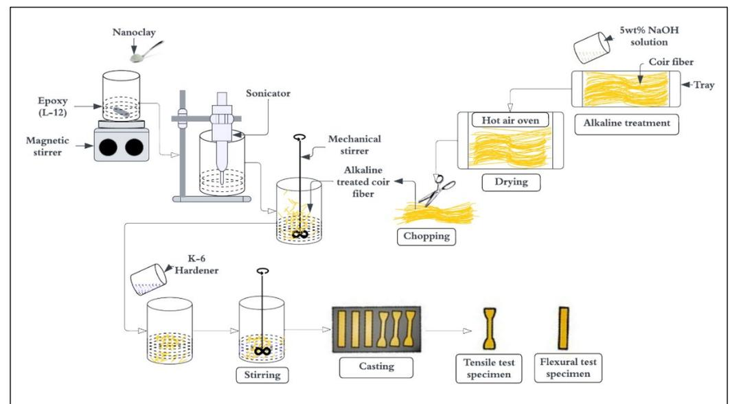
**Figure 1.** Schematic of the composite preparation technique.
