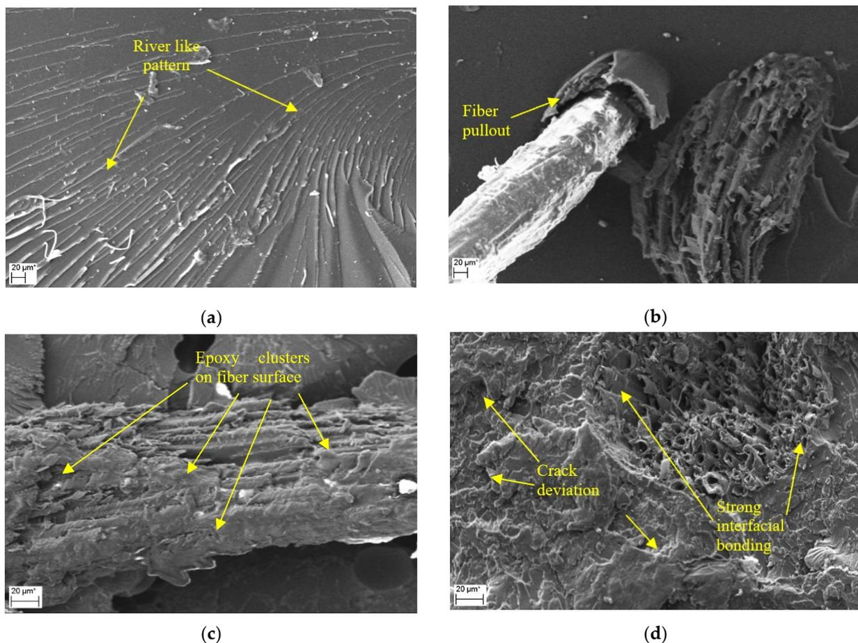
**Figure 7.** SEM images of the fractured surface of ER (a) coir fiber-reinforced epoxy composites without (b) and with nanoclay (c,d).
