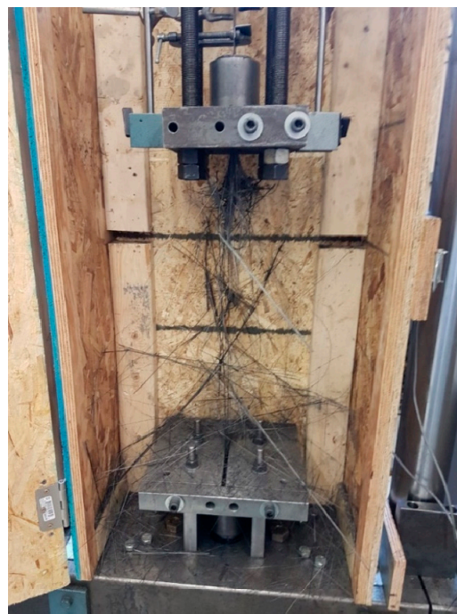
Figure 7. Fracture mode of CFRP plate outside the anchorage. Reproduced from Alhusain and Al-Mayah (2022) [38] with permission from Springer Nature.
