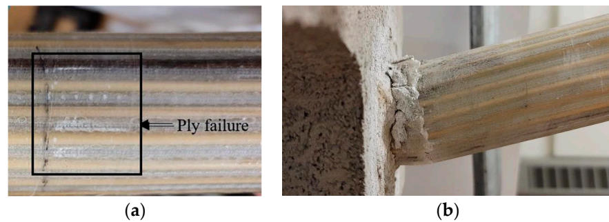
Figure 12. Typical experimentally observed (a) ply failure and (b) pole failure.
