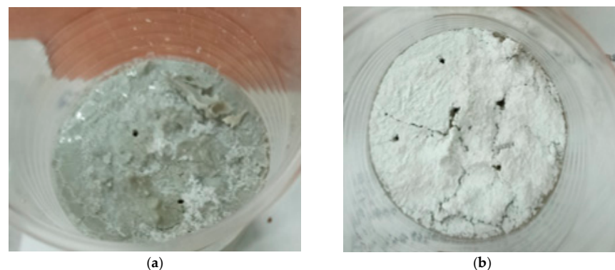
Figure 5. Efflorescence substance on the surface of mix P-CG, activated with (a) fresh alkali solution; (b) 24 h conditioned alkali solution. Treatment type—ambient conditions.
