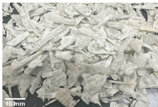
Figure 2. Thermoset matrix-coated fiber bundles.
