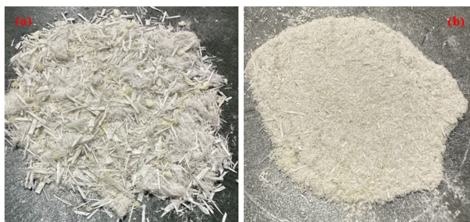
Figure 3. Appearance of EPGs after sieving for (a) coarse fiber bundles and (b) EPG powders.
