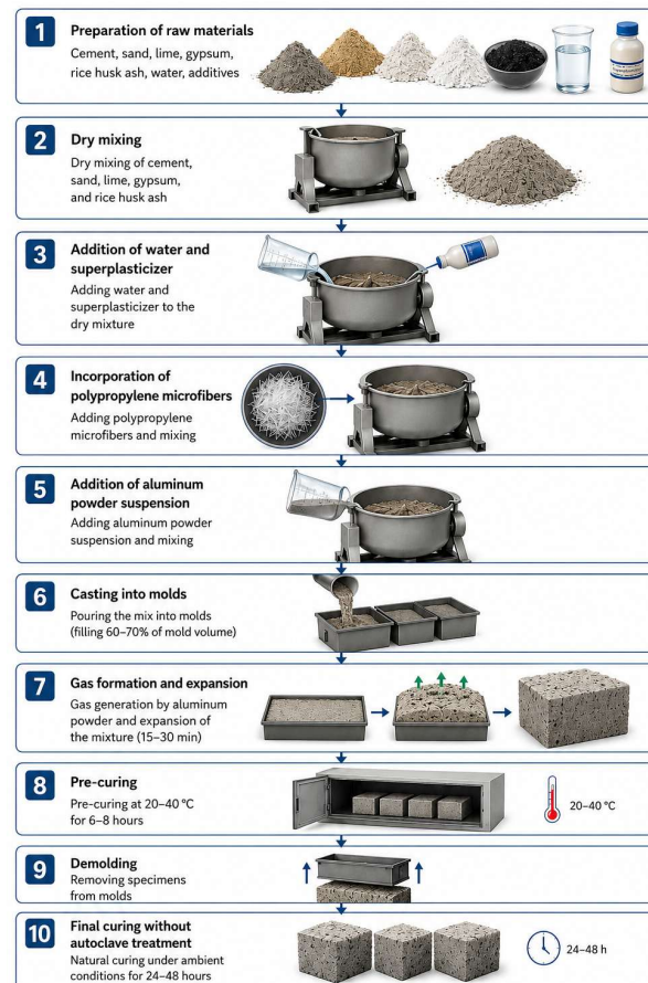
Figure 1. Technological scheme for the preparation of non-autoclaved aerated concrete incorporating rice husk ash-derived silica and polypropylene microfibers.
