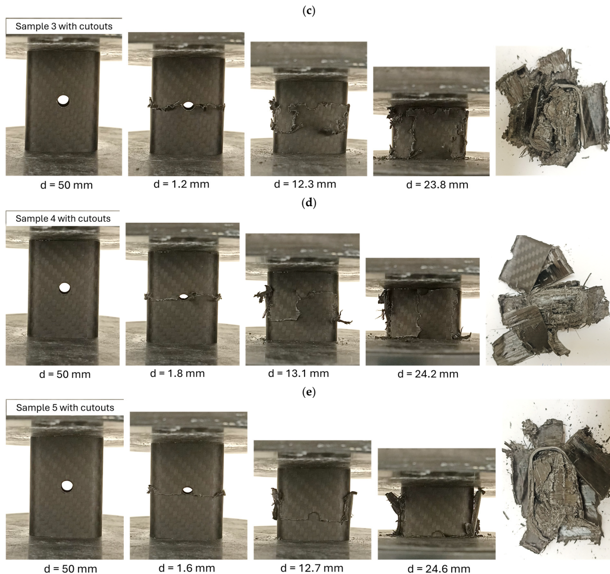
Figure 3. Failure progression of tubes with circular cutouts tubes (a) sample 1, (b) sample 2, (c) sample 3, (d) sample 4, and (e) sample 5.
