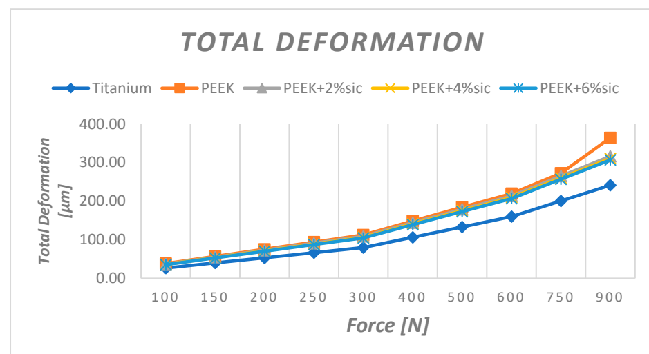
Figure 7. Total deformation (µm) for different implant materials under 45° oblique loading as a function of applied force.
