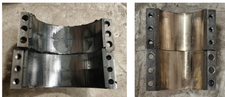
Figure 21. Wear phenomenon of the semi-metal tiles ( left ) and full-metal tiles ( right ).
