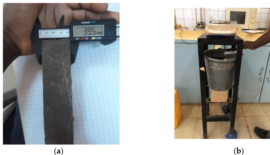
Figure 6. Instrumentation on the specimen (a) Measurement of the dimensions and (b) Hydrostatic Weighing System.
