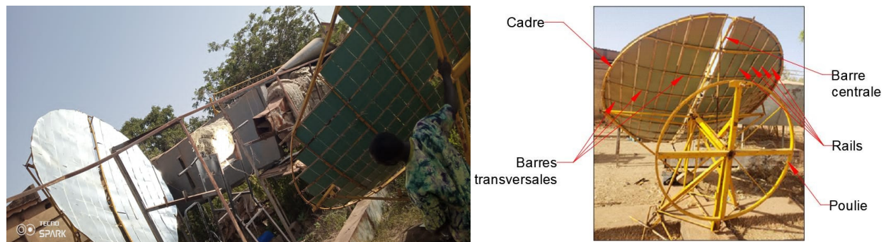
Figure 3. Layout of solar fusion device at Saaba (latitude 12.38°, longitude −1.43°).
