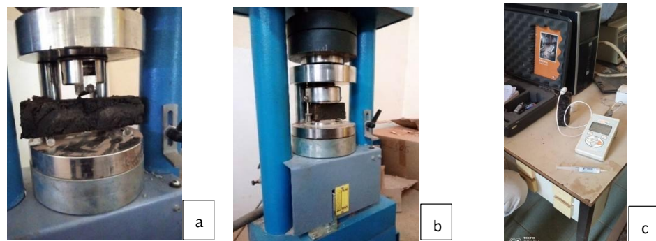
Figure 8. Experimental devices for Thermal and Mechanical tests (a) Three-point bending, (b) Compressive strength and (c) Thermal Conductivity meter KD2 Pro Decagon.
