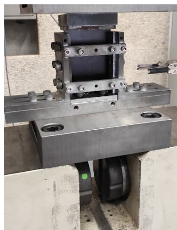
Figure 2. Experimental setup for compression after impact testing, showing the anti-buckling fixture and specimen positioning in the testing machine.
