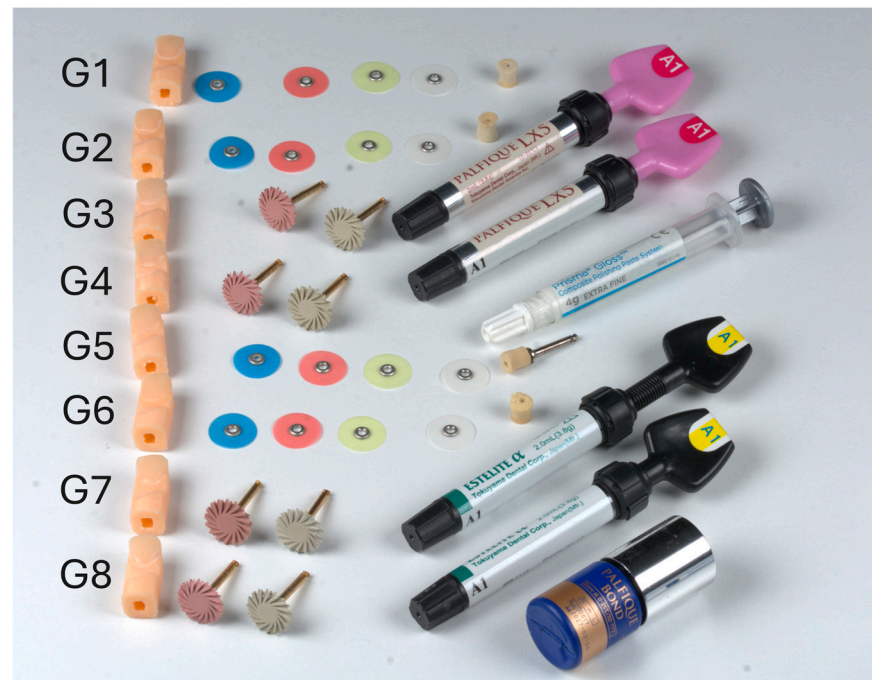
Figure 4. The experimental sample groups were categorised as follows: Groups 1 and 2 (PALFIQUE® LX5 with the standard method); Groups 3 and 4 (PALFIQUE® LX5 with the reduced method); Groups 5 and 6 (Estelite® Alpha with the standard method); and Groups 7 and 8 (Estelite® Alpha with the reduced method).
