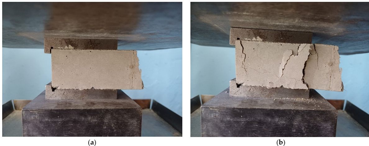
Figure 7. CS testing of half-specimens (GC): (a) before failure; (b) after failure.
