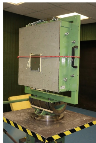
Figure 3. Clamping fixture employed for ballistic impact testing of the composite laminates.
