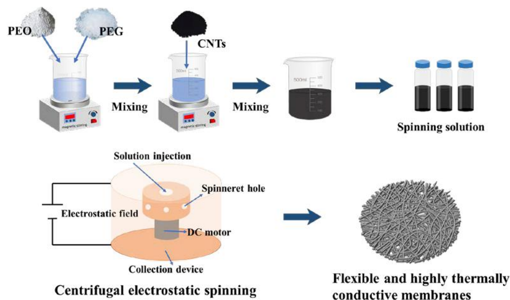
Figure 22. Centrifugal electrostatic spinning for the preparation of flexible and highly thermally conductive phase-change thermal storage membranes (reprinted and adapted with permission under a Creative Commons license (CC BY 4.0) from Ref. [261]).
