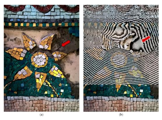
**Figure 8.** Recognition of the internal mortar structure in the mosaic sample: (**a**) Sample preparation in progress, detail of mortar application, (**b**) interferogram at 170 s after  $\Delta t = 3.1$  °C thermal excitation (80 s of excitation in a detailed acquisition) on a completed mosaic model overlaid with the photographic documentation of the sample preparation.
