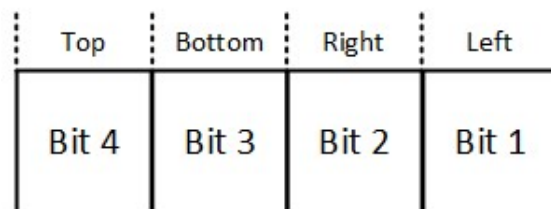
Figure 17. Outcode bits for the Midpoint Subdivision algorithm.
