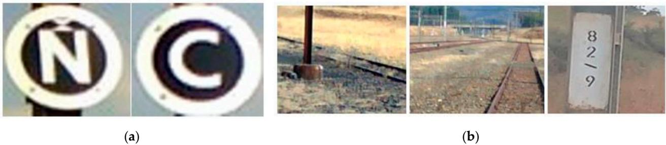
Figure 9. (a) Open (“N”) and Close (“C”) marker classes. (b) Negative image samples.
