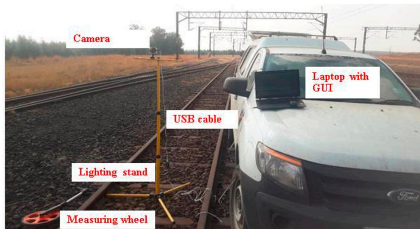
Figure 3. Experimental image capturing setup.
