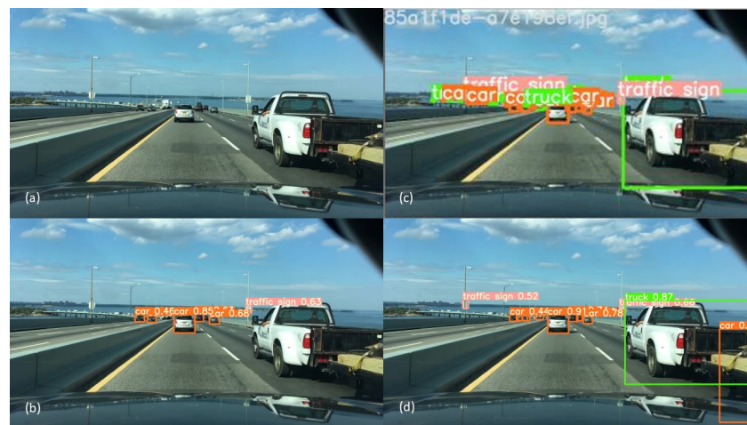
Figure 4. Example showing the effect of training with dusk/dawn data. (a)—Original image, (b)—D00N100 without dusk/dawn, (c)—ground truth, (d)—D00N100 with dusk/dawn (correctly identifies truck).
