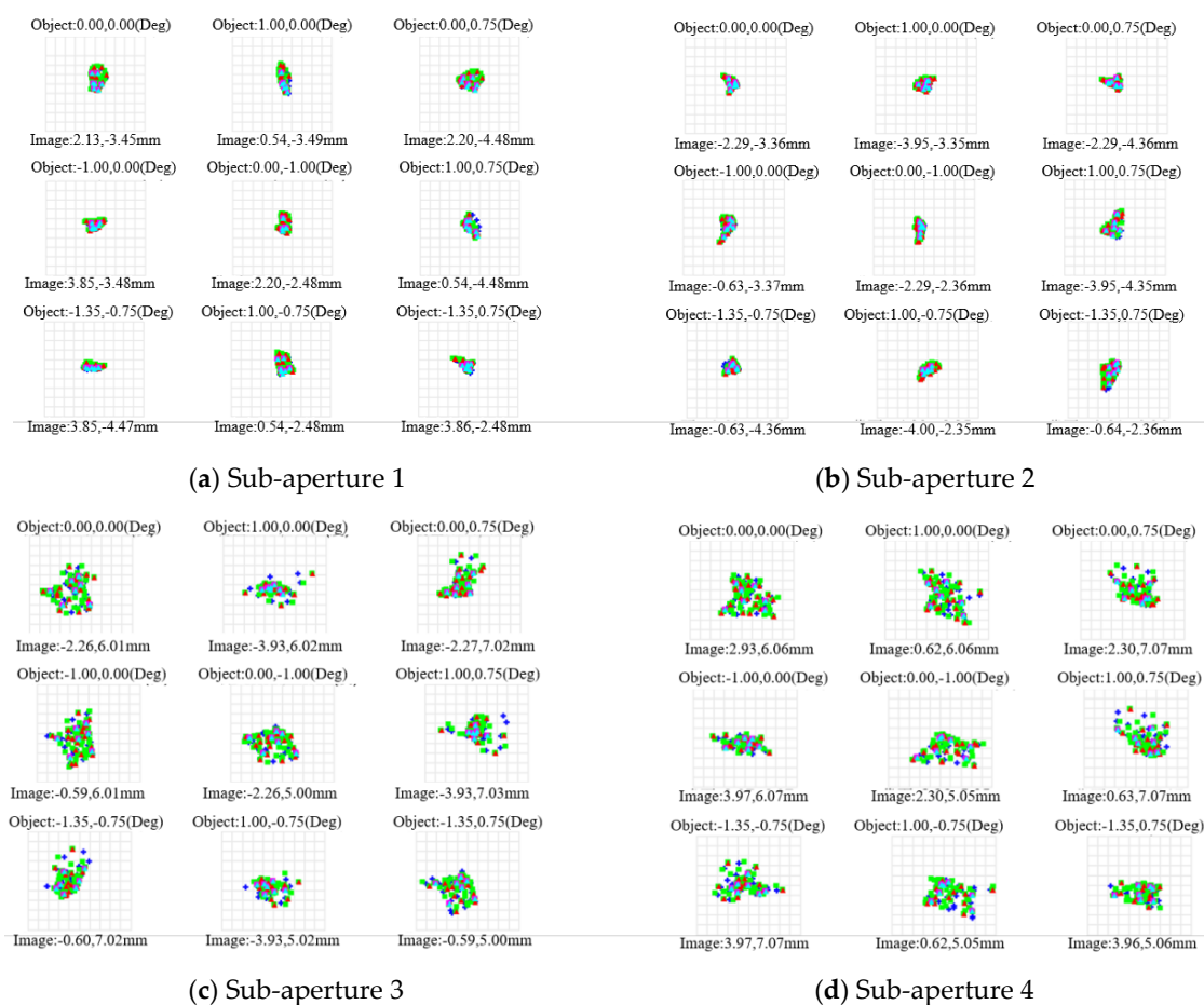
Figure 11. Spot diagram of aperture-divided off-axis simultaneous polarization super-resolution imaging optical system. (a) Sub-aperture 1; (b) Sub-aperture 2; (c) Sub-aperture 3; (d) Sub-aperture 4.
