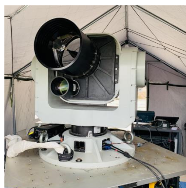
Figure 6. Physical prototype of the integrated experimental device for space target imaging, ranging, and communication.
