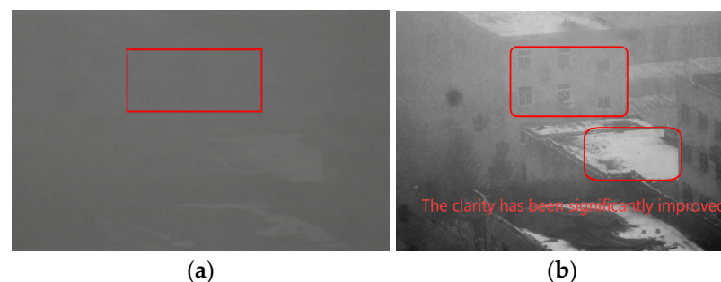
Figure 12. Passive polarization imaging of a winter scene at an imaging distance of L = 1500 m: (a) intensity imaging; (b) polarization imaging.
