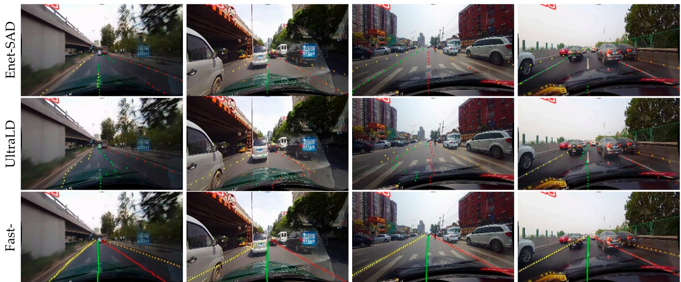
Figure 7. Qualitative comparison in lane-changing scenarios. Each row corresponds to one method: Enet-SAD, UltraLD, and Fast-CenLaneNet. Different colors indicate different predicted lane instances.
