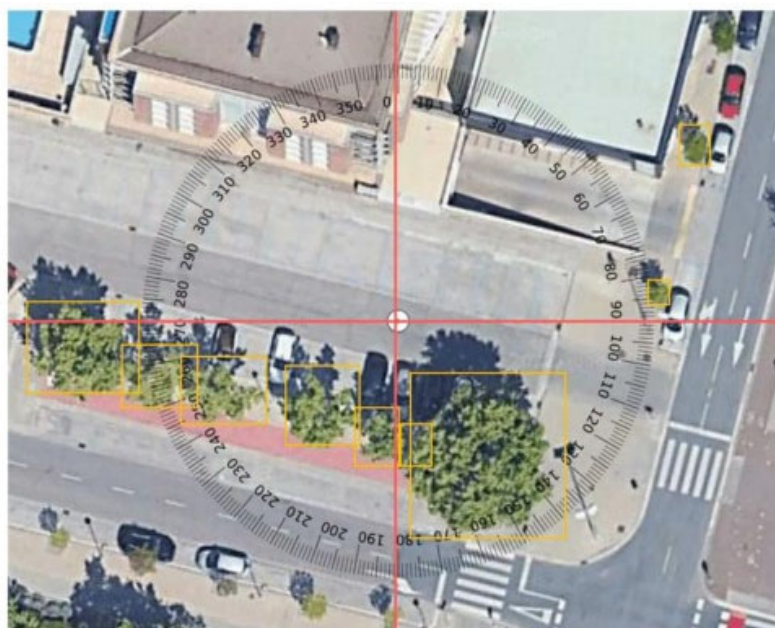
Figure 8. Example of a georeferenced spatial distribution map. Yellow boxes represent the predicted bounding box with the Deep Learning model.
