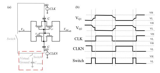
Figure 11. (a) The adiabatic schematic (b) timing signals of the adiabatic charge pump.
