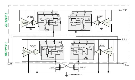
Figure 4. Proposed dual output regulating rectifier with PWM/PFM event-driven feedback control.
