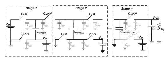
Figure 10. Linear charge pump with *n* stages.
