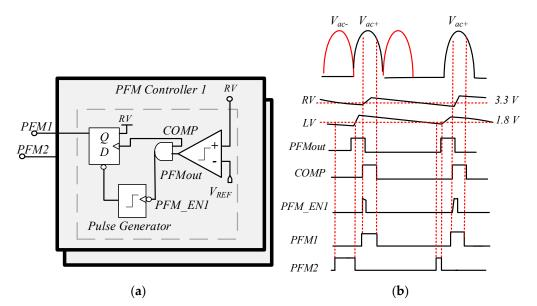
Figure 9. (a) Architecture of the PFM controller and (b) time domain response.
