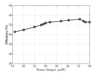
**Figure 15.** Overall system efficiency of dual output regulating rectifier and charge pump at different output powers.
