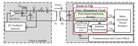
Figure 3. Proposed WPT system for a neural interface implantable device.
