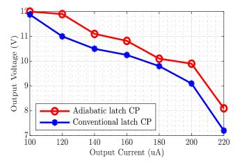
**Figure 14.** Comparison of the output voltage of the conventional and adiabatic charge pumps for 100 to 220  $\mu$ A output current. In each, the total capacitance used is 60 pF.
