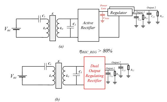
**Figure 1.** Block diagram of (**a**) conventional WPT system with *C*<sub>PASS</sub> between two stages of regulation and rectification (**b**) single stage dual output regulating rectifier.
