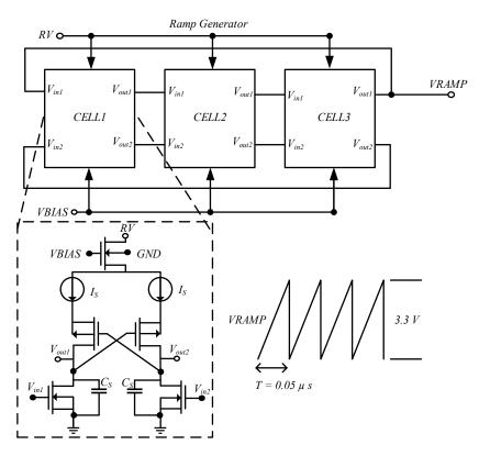
Figure 8. Accurate ramp generator circuit for VRAMP.
