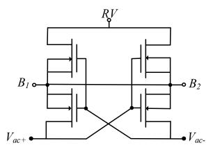
**Figure 6.** Adaptive body biasing (ABB) with  $B_1$  and  $B_2$  connected to the body of *pMOS1 and pMOS 2*, respectively.
