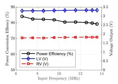
**Figure 13.** Simulated power conversion efficiency  $\eta_{PCE}$  and voltage outputs at input frequencies within the ISM band range.
