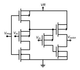
**Figure 5.** Adaptive PFM controlled buffer  $V_{PFM}$  from PFM controller, and  $V_{IN}$  from the high-speed comparator output, and  $V_{switch}$  connected as an input to the pMOS switches.
