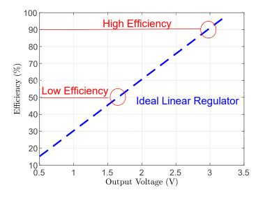
Figure 2. The LDO efficiency (Vout/Vin) of regulator changes over various output voltage.
