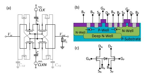
**Figure 12.** (**a**) Dynamic bulk biasing (in grey) with the charge pump design (**b**) physical implementation to the latch-up (**c**) parasitic diode between the bulk of pMOS and nMOS transistors.
