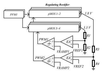
**Figure 7.** Block diagram of the dual output regulating rectifier.  $R_1$ ,  $R_2$ ,  $R_3$ , and  $R_4$  are high-value pseudo resistors. The design includes *PWM1,2* and *PFM1,2*.
