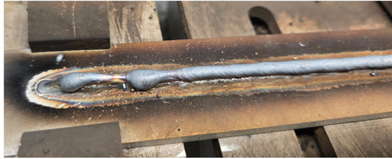
Figure 12. Corrected quality using the proposed controller in layer 2 started at low settings.
