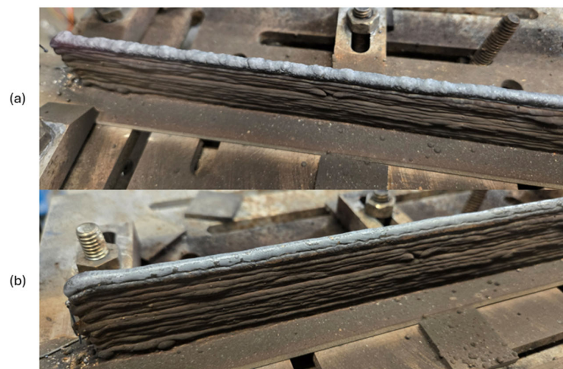
Figure 13. Corrected quality using the proposed controller in layer 13; (a) Suboptimal layer due to overcorrection, and (b) Corrected subsequent layer.
