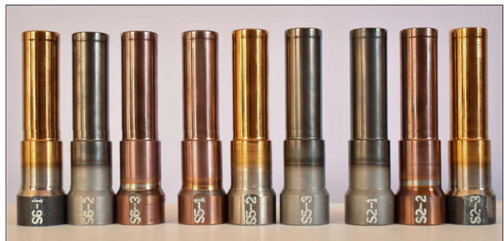
Figure 4. PVD-coated punches with the codes marked.
