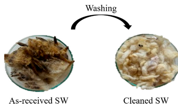
Figure 1. Photographs of the sheep wool fibers prior to (as received) and after washing.
