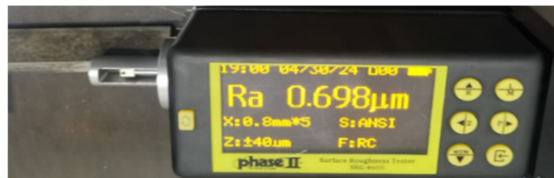
Figure 9. The calibrated surface roughness tester.
