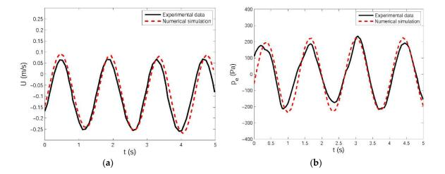
**Figure 8.** Comparison of (a) flow velocity and (b) pore pressure between the present coupled model and experimental data ( $U_0 = -0.1 \text{ m/s}$ ). The flow velocity represents the fluid velocity at 0.2 m above the seabed surface and pore pressure is from the soil element that was located at point C in Figure 7.
