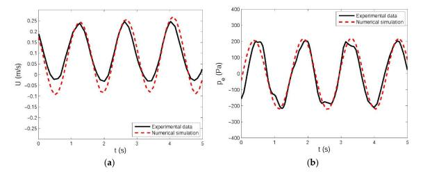
**Figure 10.** Comparison of (a) flow velocity and (b) pore pressure between the present coupled model and experimental data ( $U_0 = +0.1 \text{ m/s}$ ). The flow velocity represents the fluid velocity at 0.2 m above the seabed surface and pore pressure is from the soil element that was located at point C in Figure 7.
