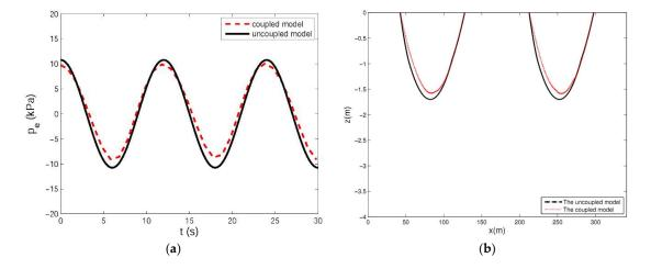
**Figure 11.** Comparison of (**a**) pore pressure and (**b**) liquefaction depth within the seabed between coupled and uncoupled models.
