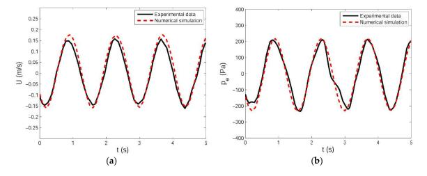
**Figure 9.** Comparison of (**a**) flow velocity and (**b**) pore pressure between the present coupled model and experimental data ( $U_0 = 0 \text{ m/s}$ ). The flow velocity represents the fluid velocity at 0.2 m above the seabed surface and pore pressure is from the soil element that was located at point C in Figure 7.
