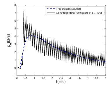
**Figure 6.** Comparison of residual pore pressure with standing wave centrifugal test data [20]. Time history of pore pressure is from the soil element at elevation z/h = 0.25.
