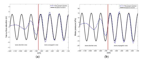
**Figure 2.** Comparison of (**a**) free surface elevation and (**b**) water pressure between the coupled model and the analytical solution. The small amplitude wave theory is applied for the analytical solution.
