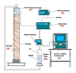
Figure 3. Schematic diagram of one-dimensional cylinder equipment (adapted from [25]).
