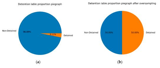
Figure 5. The proportions of classes (a) before and (b) after SMOTE processing.
