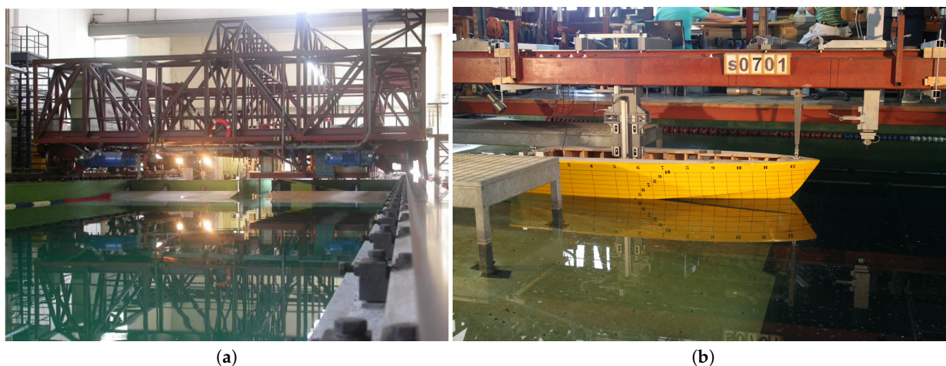
Figure 2. Front view of the towing carriage (a) and lateral view with model and towing harm (b).
