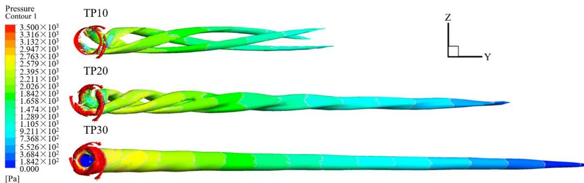
Figure 12. Vortex structure for different swirling pipes based on iso-vortex surface.
