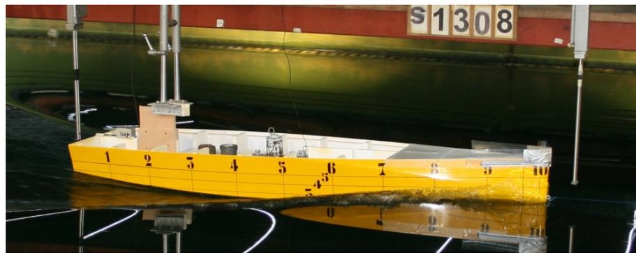
Figure 5. Scale model at  $Fr = 0.5$  tested in the Naples' towing tank.
