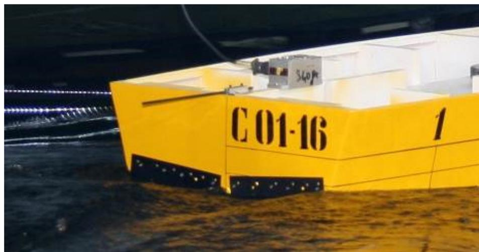
Figure 6. Detail of interceptors applied to the scale model tested in the Naples' towing tank.
