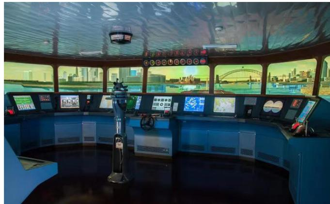
Figure 4. Full Mission Ship Handling Simulator.
