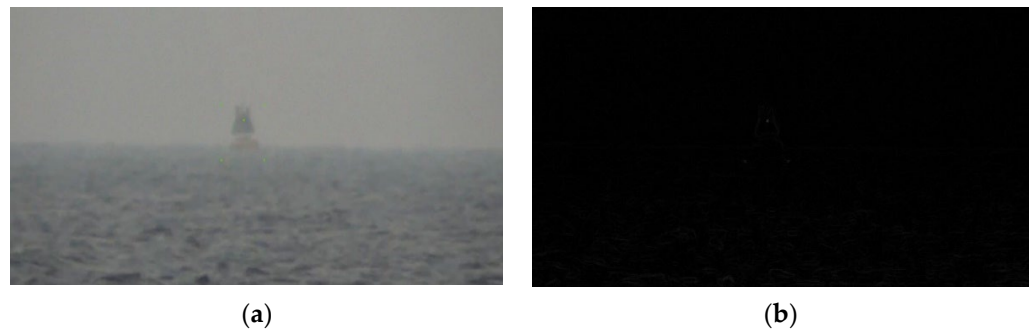
Figure 6. The extraction effect of the traditional Sobel edge detection algorithm: (a) A foggy image at sea; (b) The image extracted by the Sobel edge detection algorithm.
