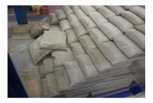
**Figure 19.** Configuration with slope 1:1.5. Uplift and movement of some elements in the stability test with H = 0.20 m, T = 1.5 s and h = 0.40 m.
