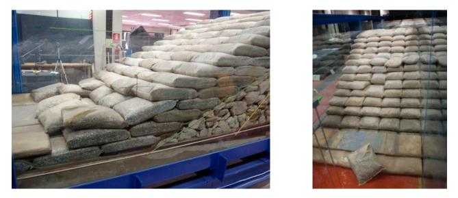
**Figure 20.** Configuration with slope 1:2. Sliding of some elements in the stability test with H = 0.20 m, T = 2.0 s and h = 0.40 m (**left panel**) and removal of elements in the stability test with H = 0.20 m, T = 3.0 s and h = 0.40 m (**right panel**).
