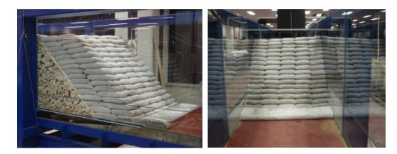
Figure 5. GSC revetment structure with a slope of 1:1 (lateral and front views).
