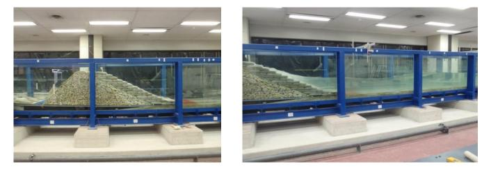
Figure 6. GSC revetment structure with a slope of 1:2.
