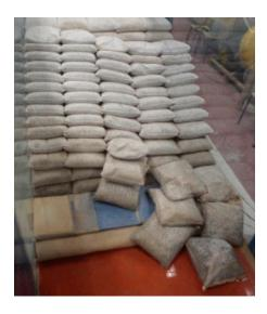
**Figure 18.** Configuration with slope 1:1. Instability of the structure in the stability test with H = 0.20 m, T = 2.0 s and h = 0.61 m.
