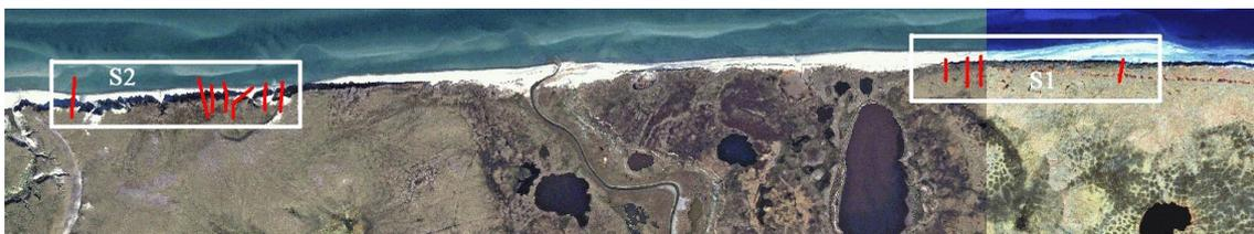
**Figure 10.** The study area consists of two sites, S#1 and S#2, with distinct bluff height differences. S#1 consists of low bluff heights. Coastal profiles are shown with red lines. Image source: Internal reports, SAMCoT.
