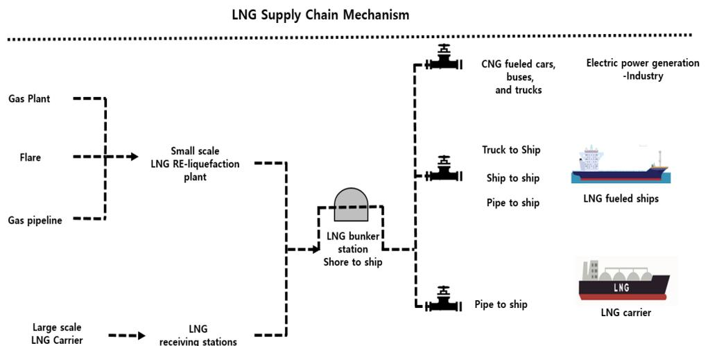
**Figure 3.** LNG supply chain overview. LNG, liquefied natural gas.
