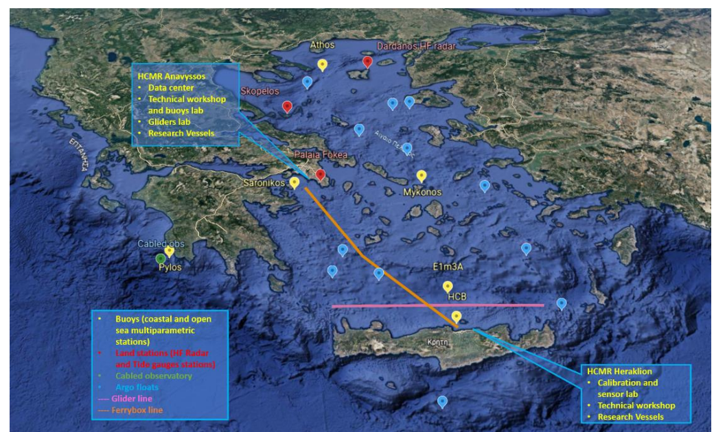
Figure 2. The POSEIDON system operational nodes and shore facilities.
