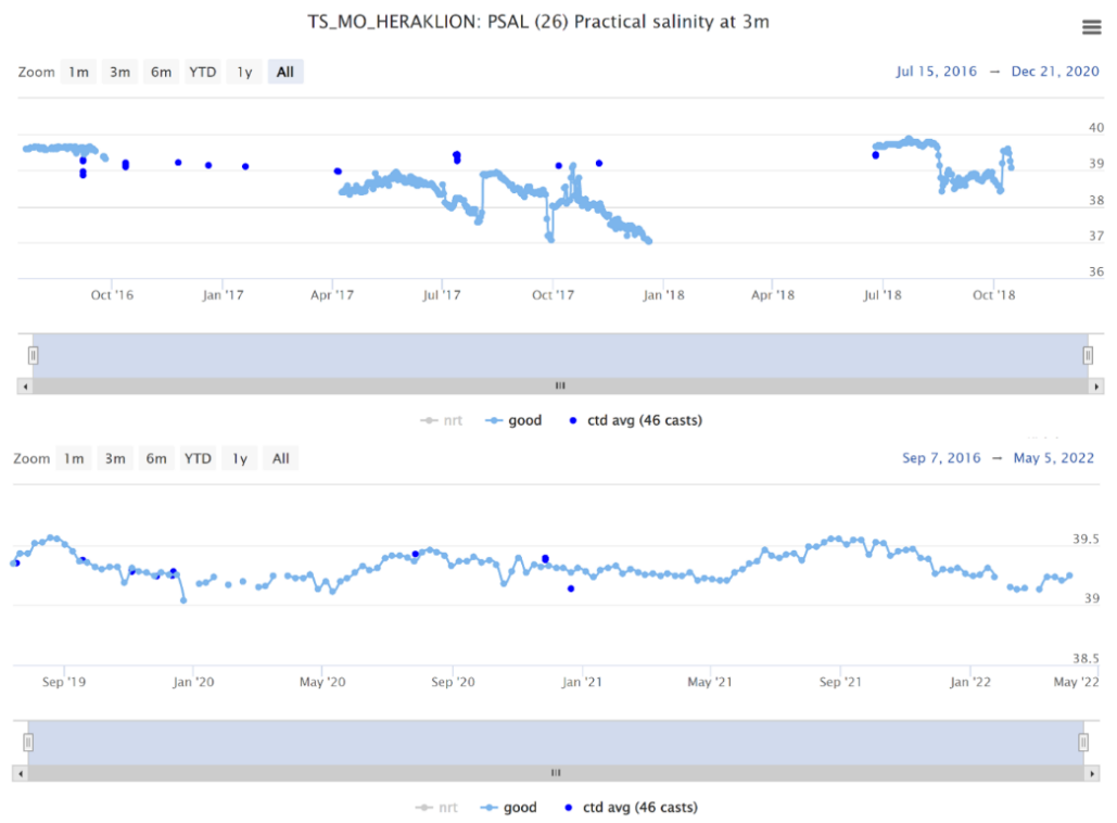
Figure 11. The improvement of the salinity measurements after the replacement of the exposed surface sensor with one equipped with a pump and a flow-through system proven to be more effective against fouling.
