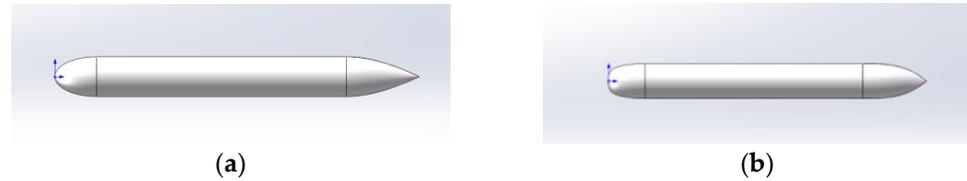
**Figure 7.** Three-dimensional sketch of two kinds of hull models, the model with  $p = 2; \theta = 25^\circ$  (a) and the model with  $p = 4; \theta = 40^\circ$  (b).
