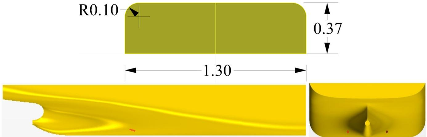
**Figure 5.** Geometry of FCF and 3D views of hull with FCFs attached.
