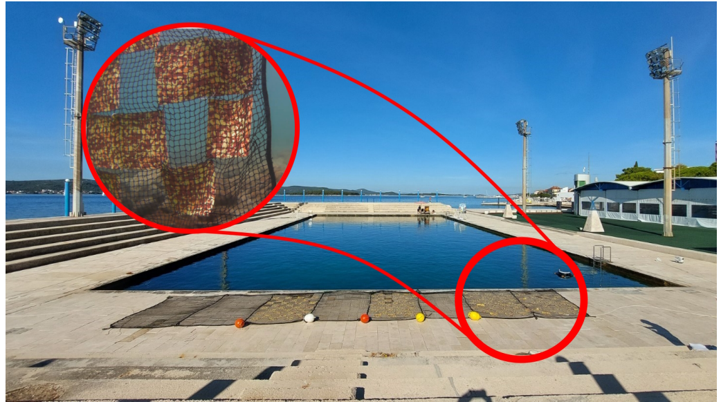
Figure 10. The Olympic sea water pool used for testing, with the net dragged out in order to place patches for biofouling simulation. The affixed patches on the net can be seen close-up filmed during a mission in the red circle.
