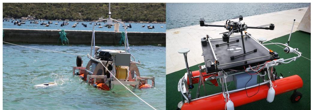
Figure 2. Autonomous surface vehicle Korkyra: (left)—TMS mounted, (right)—LP mounted onto the ASV.
