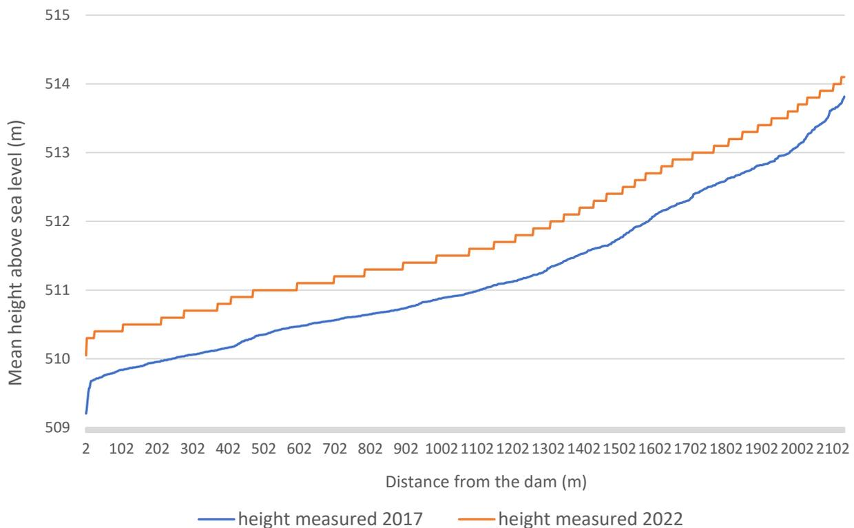
**Figure 7.** Comparison of seabed elevations measured in the 2017 survey (blue) and 2022 survey (orange).
