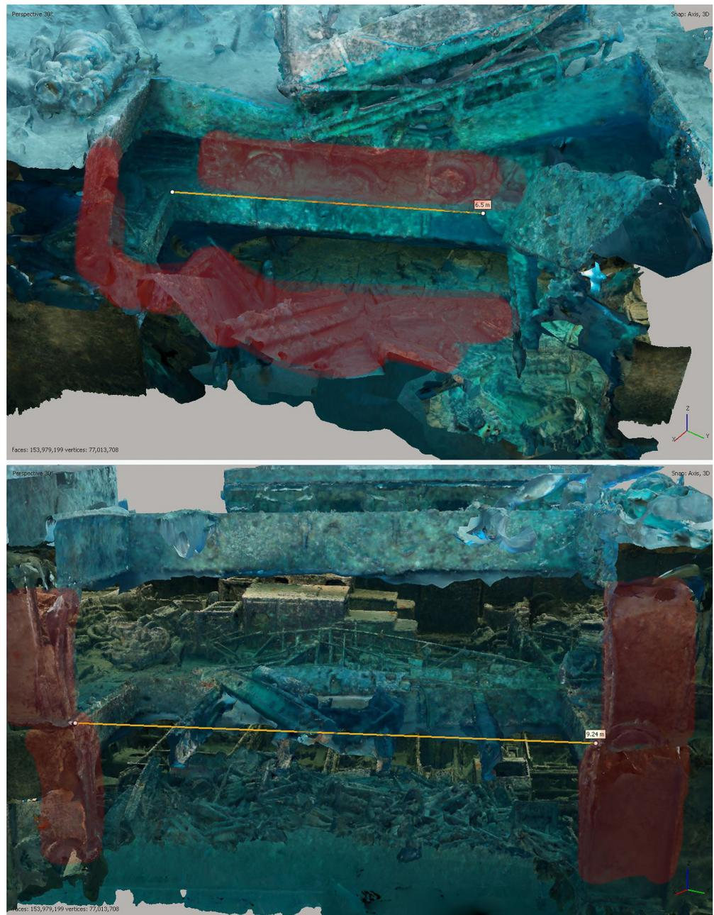
**Figure 5.** (Top): Section through Hold No. 1 viewed from starboard side with red highlight showing areas requiring care to ensure overlap between the main, upper, and lower cargo decks. The partial collapse of the main deck on the port side has provided plenty of material. (Bottom): Section through Hold No. 2 viewed from the starboard side. The red areas highlight vertical supports between decks.
