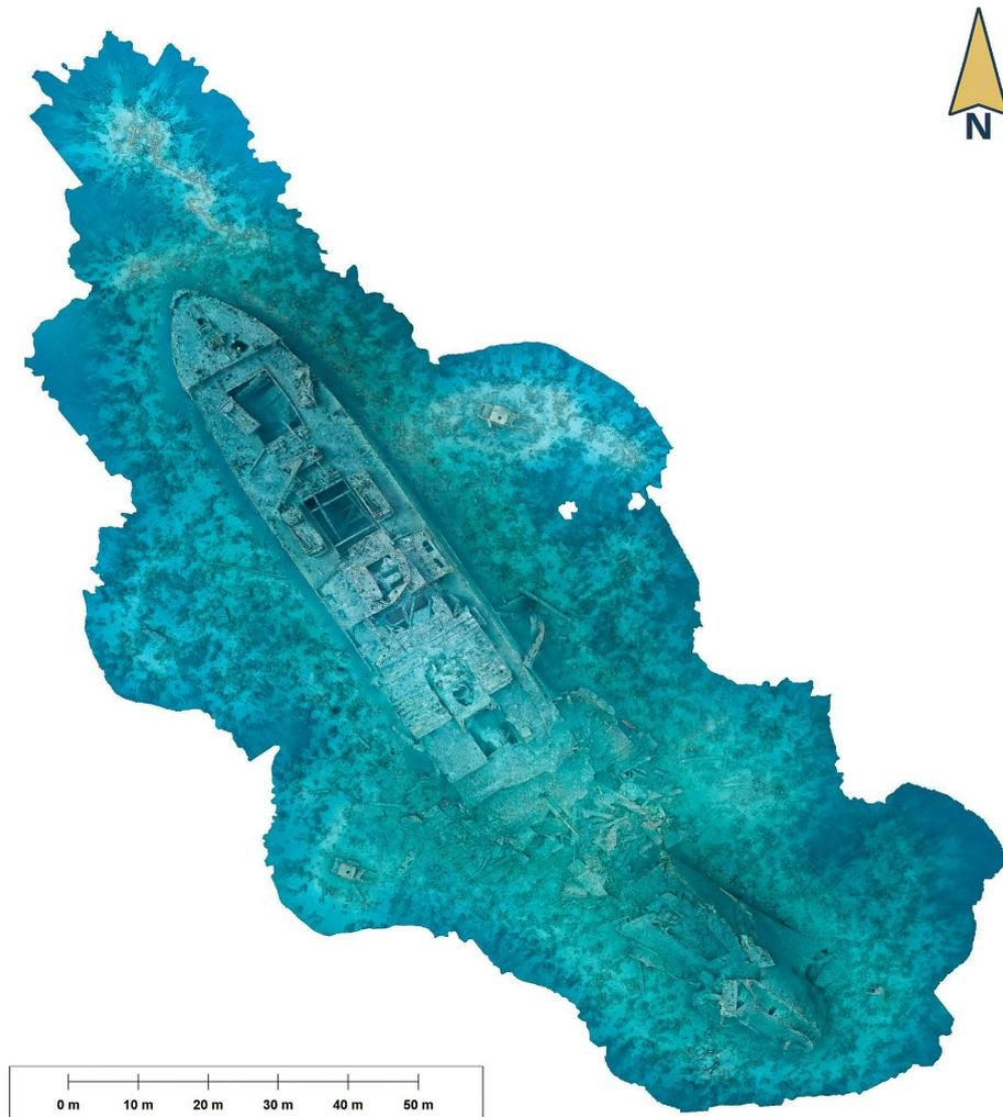
**Figure 2.** Orthophoto derived from the 3D model of the SS *Thistlegorm*. Here, the wreck and surrounding seabed are viewed from the surface. The main deck from bow to just aft of the engine room have been well preserved. The explosion centered at Hold No. 4 has completely destroyed the ship in this section. The stern, now lying on its port side, remains preserved.
