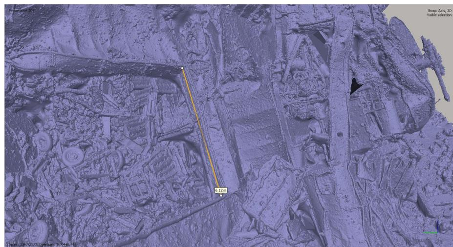
**Figure 22.** Measurement across the lower deck of Hold No. 5 entrance used to confirm model accuracy.
