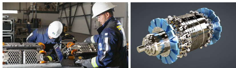
Figure 13. PAUT ILI tool from NDT Global and Trapil.
