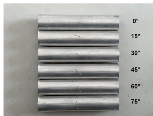
Figure 18. The test tubes in the damaged liquid-filled cylindrical shell crack propagation experiment.
