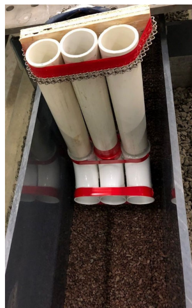
Figure 5. Injection tubes across the channel's width.
