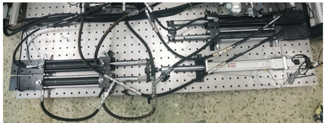
Figure 20. Schematic diagram of 1/2 parallel interconnected suspension.
