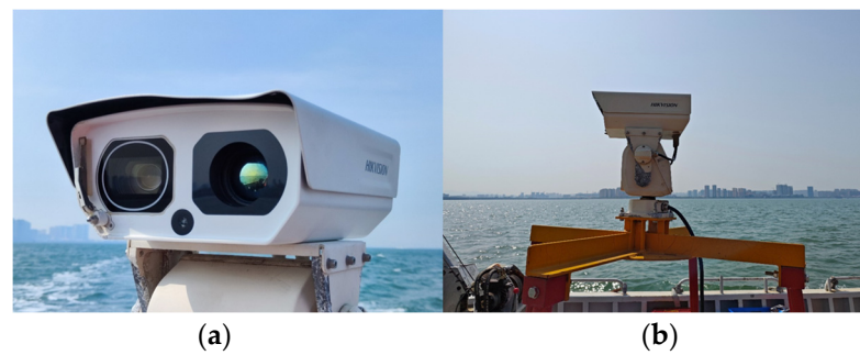
Figure 1. (a) HIKVISION camera; (b) capture bracket.
