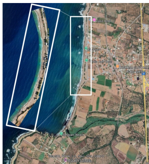
Figure 2. Reconstruction of the coast of Kalo Nero, Greece, using images from the drone survey.
